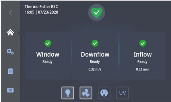
**Figure 4-12.** Main Screen - Unit working
