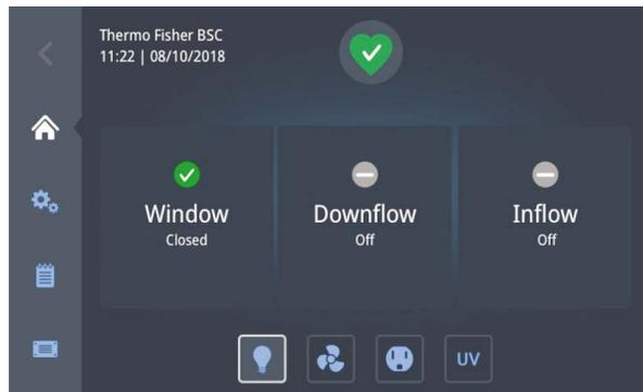
**Figure 4-14.** Main Screen - Unit in Idle Mode, window closed
