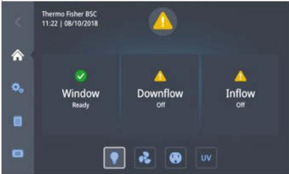
Figure 4-15. Main Screen - Unit in Idle Mode, window ready
