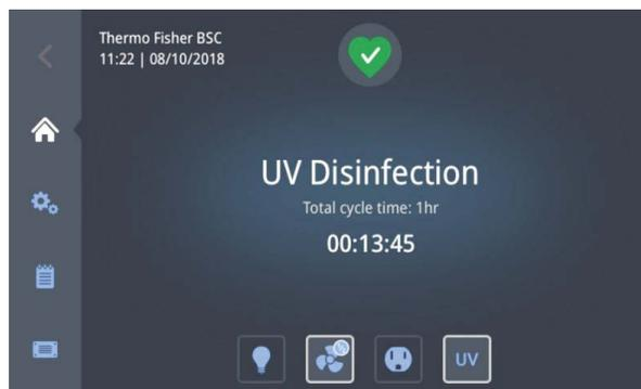
**Figure 4-18.** Main Screen - “UV disinfection” running
